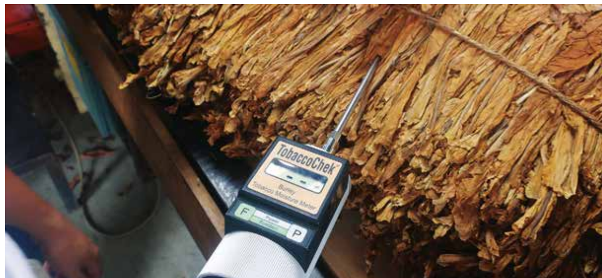
When receiving tobacco bales from farmers the tobacco is graded and moisture content is assessed.
